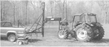
Pickup-mounted lift gets people into almost any machine, eliminating the need to alter each piece of equipment. Unit rotates 180 degrees and reaches out 8 ft. and up as high as 10 ft.
