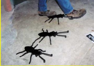
Your readers may get a kick out of the boot jacks I make that look like giant metal bugs. They're made of heavy plate steel and bent rod. I built a jig to hold all parts prior to welding them into place. The bugs sell for \$35 apiece. **(William Winter, Rt. 2, Box 80, Tower Hill, Ill. 62571 ph 217 567-3191)**
