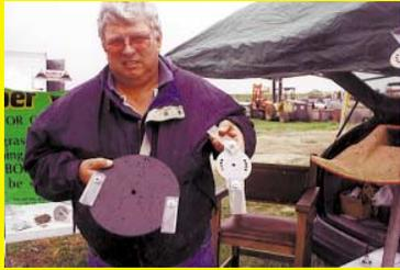
blades that are very light in weight and super strong and long wearing. They can be resharpened with a grinder or a file.
