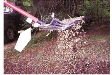
Arrow points to small electric motor that shakes tines on fork.
