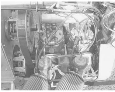
Hasbrouck's 126 Cub Cadet garden tractor is equipped with 31-in. rear "pulling tires". Tractor is powered by a custom built 2-cylinder, 2-cycle engine with just under 200 hp.
