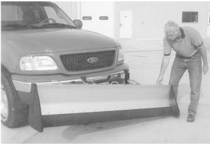
To attach plow, you lift one end of blade at a time over a pair of vertical holders mounted on a push frame. Frame slides into a receiver hitch on front of vehicle.
