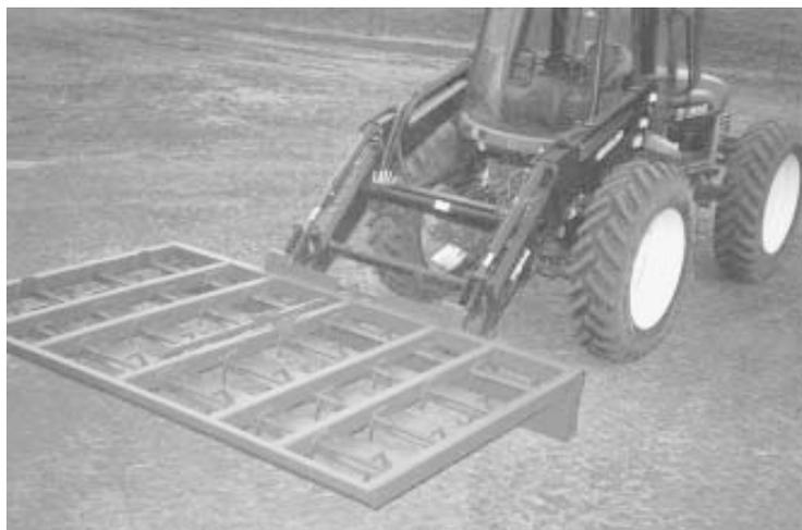
**Schmidt made a quick-tach hitch for his bale fork, allowing him to use it on either his New Holland TR 140 Bi-Directional tractor or his Allis 8050 front wheel assist tractor.**
