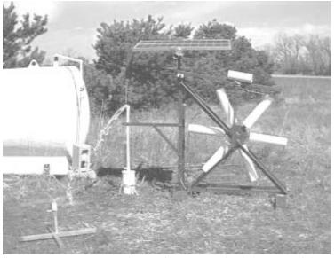
Solar-powered pump has a walking beam/rocker arm design similar to that of oil well pumps. Concrete-filled flywheel kicks in at 40 rpm's to boost efficiency.
