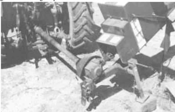
Jacobs replaced auger's original pto driveshaft with a right angle gearbox.
