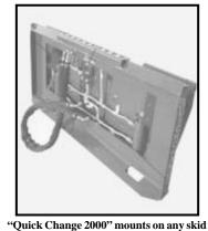
loader equipped with universal quick tach mounting brackets and is equipped with a pair of spring-loaded pins operated by hydraulic cylinders. It eliminates the need to get out of the cab and manually latch or unlatch pins.
