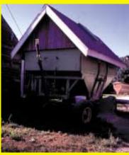
I converted a Parker 200-bu. gravity wagon to hold feed for my sows. To keep out rain and snow, I put a roof on the wagon. It was less expensive than buying a commercial tarp and it will last longer.
