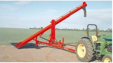
The "grain pile" auger is equipped with a 13-in. dia. auger that has a 5 1/2-ft. wide sweep hopper at its bottom end. Hopper is designed to float and follow ground contour.
