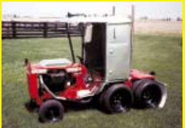
dual wheels all the way around. It resembles a Peterbilt semi tractor, but I call mine a CharlieBilt. I made it out of a pair of Wheel Horse 70 tractors. I use it to pull a 12-ft. long, 40-in. wide flatbed trailer equipped with a plywood floor. A fifth wheel hitch mounts behind the tractor.
