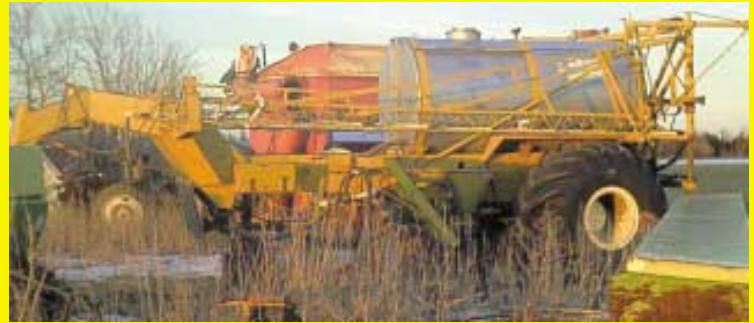
I took a Big A sprayer with a blown engine and turned it into a gooseneck sprayer that I pull with my tractor. It has a 1,200 gal. stainless steel tank. I took the cab, motor and transmission out. A local welder made a gooseneck for it. I put a hydraulic motor on the frame to run the Scott pump that was already on the machine. I didn't have to move the pump.
