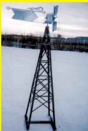
This is an ornamental windmill I made from angle iron and flat iron. I fitted it with an alternator and fan from an old car. I removed the brushes and regulator which allows the alternator to turn easily. (**Pete Peters, Osler, Sask.**)
