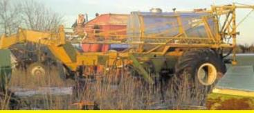
I took a Big A sprayer with a blown engine and turned it into a gooseneck sprayer that I pull with my tractor. It has a 1,200 gal. stainless steel tank. I took the cab, motor and transmission out. A local welder made a gooseneck for it. I put a hydraulic motor on the frame to run the Scott pump that was already on the machine. I didn't have to move the pump.
