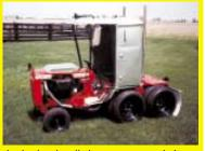
dual wheels all the way around. It resembles a PeterBilt semi tractor, but I call mine a CharlieBilt. I made it out of a pair of Wheel Horse 70 tractors. I use it to pull a 12-ft. long, 40-in. wide flatbed trailer equipped with a plywood floor. A fifth wheel hitch mounts behind the tractor.
