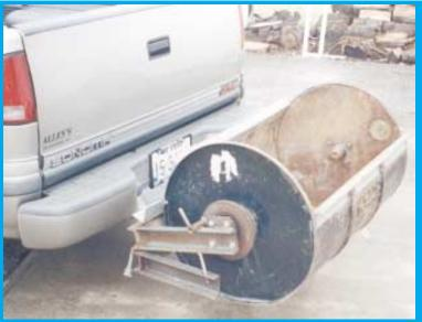
Henderson mounted auto hubs in the center of each end of a 55-gal. metal drum. Frame slips into pickup's receiver hitch.
