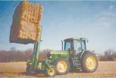
Bale handler attaches to tractor frame by parallel linkage and is supported by two independent castor wheels.
