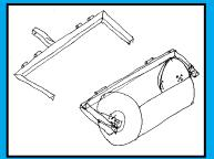
U-shaped channel iron frame wraps around back and each end of drum.
