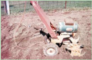
Bob Unger replaced the original gas engine on his rototiller with a 1 hp electric motor. "I've used it for 10 years and I've never cut a cord," he says.
