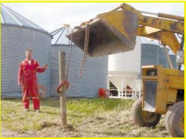
Simple post puller uses a 14-in. dia. pressure plate off an old clutch. Allard welded one end of a chain to edge of plate and hooks the other end to his front-end loader.
