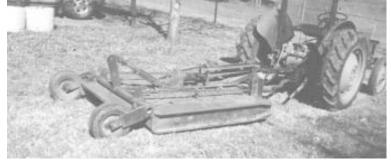
Pto-driven, drawbar-pulled mower was built out of an old military truck frame and other miscellaneous parts. It cuts a swath 5 ft. wide.
