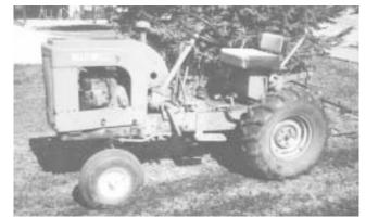
Deere "L" look-alike is powered by a 20 hp, 2-cyl. engine off an old pull-type combine.
