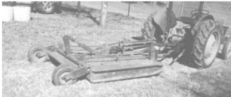
**Pto-driven, drawbar-pulled mower was built out of an old military truck frame and other miscellaneous parts. It cuts a swath 5 ft. wide.**
