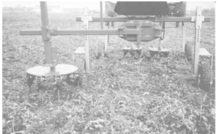
Pto-driven weeder wheels are equipped with rubber fingers, which uproot weeds without damaging the crop.
