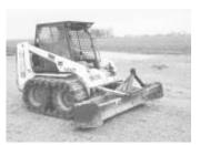
Wessling also modified an 8-ft. wide, 3-pt. mounted box blade so it quick-taches to skid loader.
