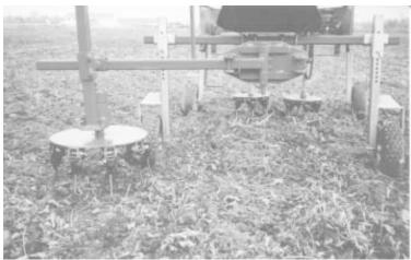
Pto-driven weeder wheels are equipped with rubber fingers, which uproot weeds without damaging the crop.
