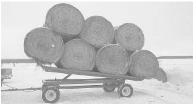
Simple flatbed bale hauler simply dumps bales off the back to unload.
