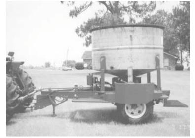
Randy Thompson's machine is equipped with a stainless steel, hopper-bottom fertilizer mixer tank. Infrared sensors help fertilize two rows of trees at once.
