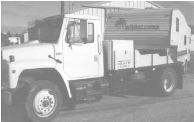
Robert Ellis converted a 1985 IH 2-ton moving van into this dually pickup that's equipped with a fifth wheel hitch on back. "I saved a lot of money compared to buying a new 1-ton pickup," he says.
