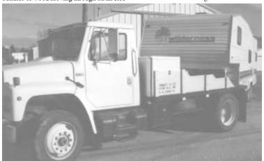
Robert Ellis converted a 1985 IH 2-ton moving van into this dually pickup that's equipped with a fifth wheel hitch on back. "I saved a lot of money compared to buying a new 1-ton pickup," he says.
