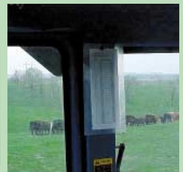
Chart in tractor cab is used to convert pounds of pressure to pounds of hay.
