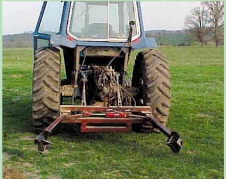
Pattie's weigh scale mounts on 3-pt. bale unroller. He filled the top link hydraulic cylinder with fluid and then ran a hose into a 600 psi pressure gauge. Bale exerts pressure on top link, which affects pressure reading.
