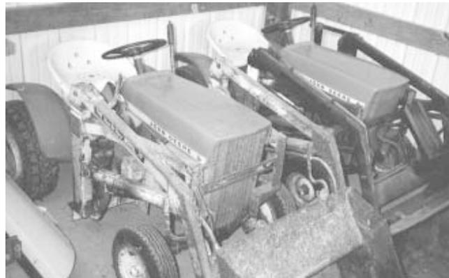
His rarest model is a 1965 Deere 110 equipped with a trip rope front-end loader. A model equipped with a hydraulic dump loader is shown at right.
