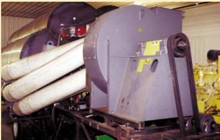
Prototype in-field dryer allows hay to be dried right in the field. The multi-chambered, pull-type machine measures 45 ft. long by 12 ft. wide and about 12 ft. tall.
