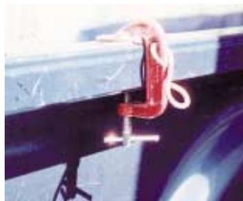
Tie-down bracket is made by brazing a flat washer to “fixed” end of clamp, then drilling a hole in clamp and inserting an S-hook that’s closed into a loop.
