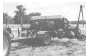
**Julian Huffman mounts his IH 800 3-pt. planter on the "caddy" made out of a semi trailer axle, which is equipped with a 10-ft. long hitch.**
