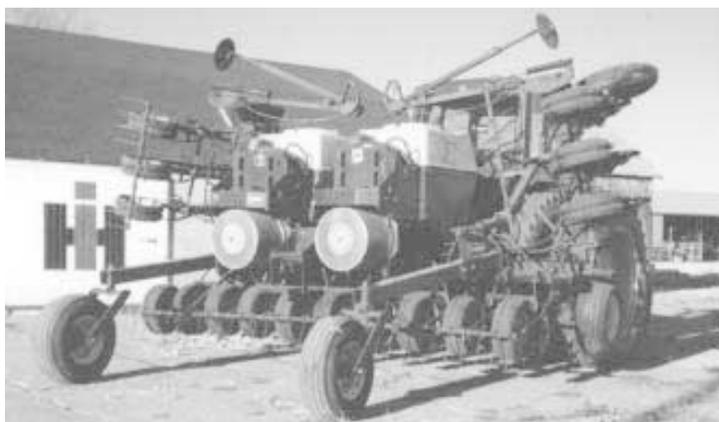
**Nieman built his 16-row, 16-in. soybean planter (above) out of two used IH 500 Cyclo air planters. He added Keeton seed firmers to Acra-Plant shoes (right) to keep seed from bouncing out of the ground.**
