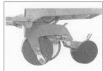
**Steel holder bracket is held with wear blocks rigidly to shank just ahead of seed tube.**
