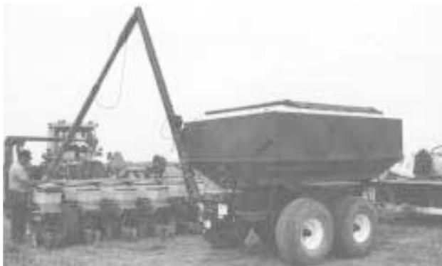
**Tandem axle seed loading unit is complete with a hydraulically-operated auger and 15-ft. telescoping downspout.**
