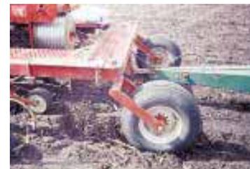
To split the rows made by the IH planter, Neubauer offset the row units on the Deere planter and mounted a hitch on back of the IH planter.
