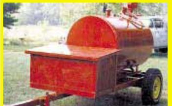
leave it there. It saves a lot of tractor riding back and forth just to get gas. The tank is a standard 500-gal. fuel tank that mounts directly over the axle, which came off a pickup. An inexpensive hand-
