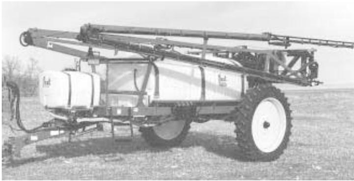
Fast's new spray boom pivots at the center to always keep boom parallel to ground.
