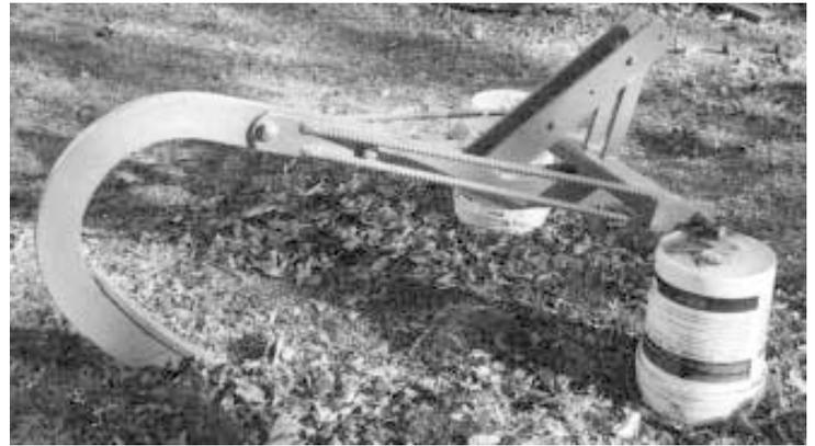
Seltzer made this 3-pt. "subsoiler" out of an old Allis-Chalmers belly-mounted subsoiler. He built it last spring after he had problems with water standing on headlands.
