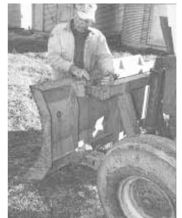
Home-built mounting brackets are hinged to allow blade to move up and down.
