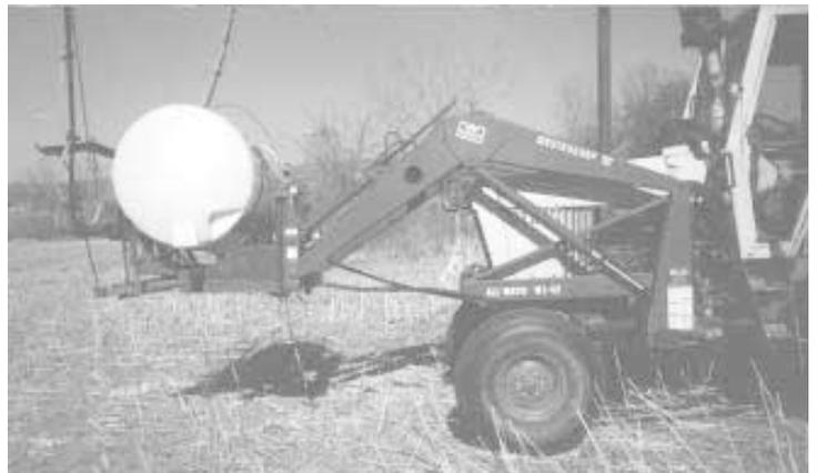
All components mount on a Case 1175 tractor equipped with a heavy-duty front end.
