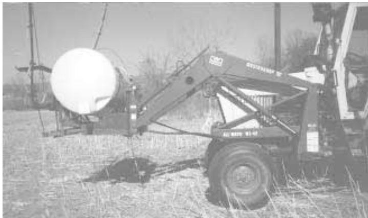
All components mount on a Case 1175 tractor equipped with a heavy-duty front end.
