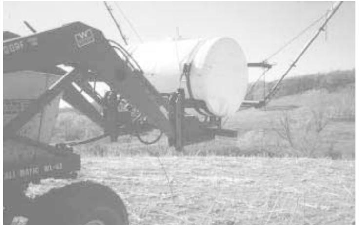
The Barbers used the booms, pump, and tanks from their existing trailing sprayer, mounting the tanks on either side of a steel frame salvaged from a pull-type sprayer.
