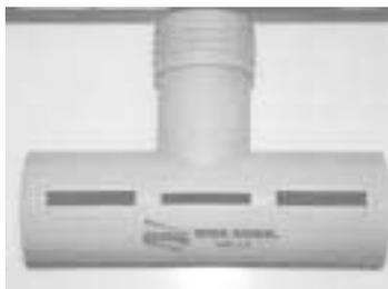
The 6-in. long, T-shaped, PVC unit has three slots in it. Foam squeezes out of slots in flat, narrow ribbons that cover a total width of about 6 in.
