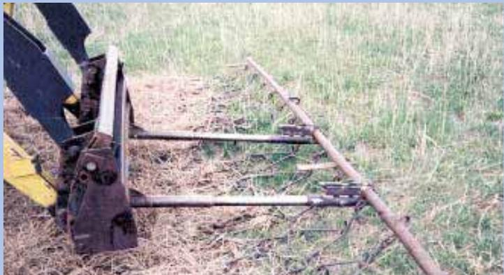
He attached harrow to his front-end loader using Farmhand quick-attach shafts designed to carry pallets. A pair of pipe sleeves slip over the two Farmhand shafts.
