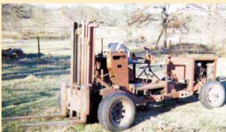
To see the rear-mounted forklift, Eddings moved the seat, steering wheel and controls 90 degrees to the right, so driver faces passenger side.
