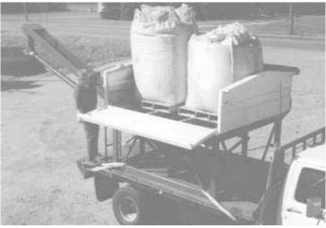
One side of hopper can be folded down, allowing you to use a forklift to set two 2,500-lb. bulk seed bags or two "Pro Boxes" into hopper.
