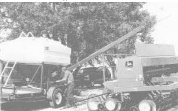
Swinging conveyor allows you to fill up to a 20-ft. planter without having to move unit. Conveyor mounts at base of steel hopper that mounts on any trailer or truck flatbed.
