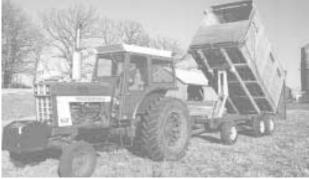
Wagon is raised and lowered by a 10-ton hydraulic cylinder that operates off tractor hydraulics. Works great for filling bunker silos.
