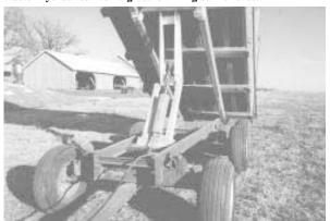
Wagon is hinged at back where it raises up and has a reinforced frame.
