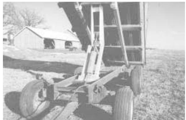
Wagon is hinged at back where it raises up and has a reinforced frame.
