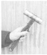
an inexpensive, heavy hammer. The shaft had been accidentally bent. I cut off a length of the shaft and burned a hole through it. I used a length of sq. steel tubing to make the handle and butted the two pieces together, then ran a bolt through the shaft and tubing and fastened a nut to the bottom of the bolt."
