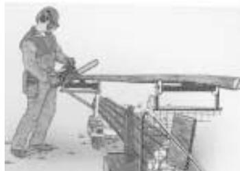
**Unit can be used to pull a cart equipped with a pair of rollers that can be used to hold logs for cutting.**
