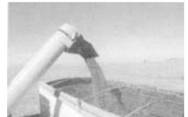
**Spout extends the reach of the auger by 24 in. and then directs grain straight down into truck or cart. It fits all 10 to 14-in. dia. top and bottom swing augers.**
