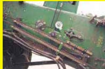
Deere's CTS combine is supposed to be the Cadillac of combines but the farmer who owned it said the dust reducer wasn't getting the job done. We pulled Deere's unit out of the feederhouse and covered the hole with steel plate, then mounted the E-Z View on top of the feederhouse. We belt-drive our unit off the original drive for Deere's unit. Our customer is happy with it.
