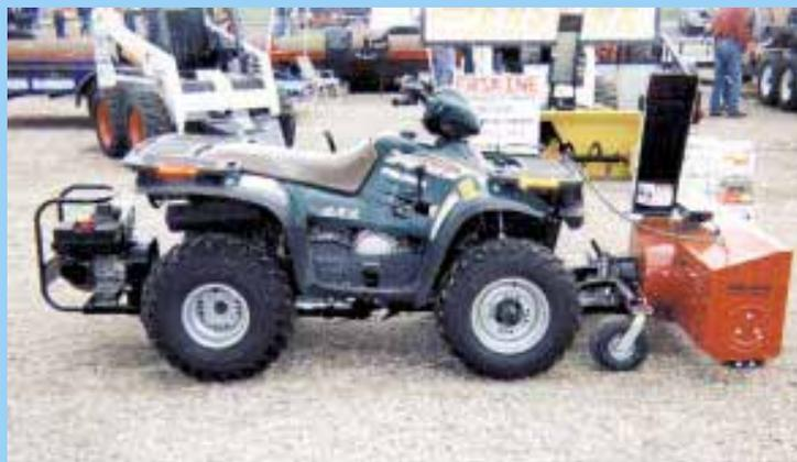
Rear-mount engine helps balance the snowblower's weight, making the ATV easy to steer at all times.
