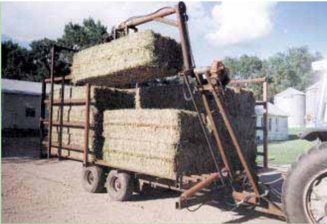
As worm-drive gearbox rotates arm up and over the wagon bed, a grapple fork places the big square bale on the load.
