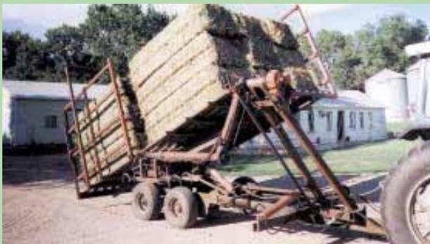
Hoist slides first tier of bales to rear during loading and later deposits entire stack for storage. Grapple hooks tuck beside wheels during transit.
