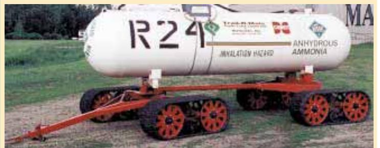
New "Trail-R-Mate" tracks are designed to mount on non-powered implements, such as this anhydrous ammonia running gear.
