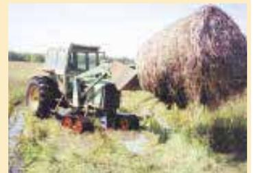
The 16-in. wide tracks can be used to replace the front wheels on 2-WD tractors.
