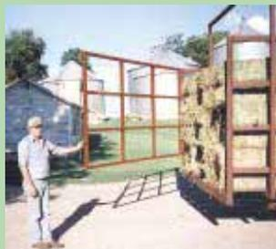
Operator can swing the endgate free allowing the stacked bales to slide free of the wagon when the hoist is engaged.
