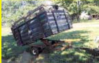
I used sq. tubing to make a subframe for the trailer and mounted a 4 by 24-in. hydraulic cylinder on it. The cylinder is powered off the hydraulics that operate the snowplow attachment on front of the riding mower. The box measures 8 ft. long, 5 ft. wide, and 4 ft. high and has plywood sides so it's very lightweight. A metal screen across the tailgate allows exhaust air to escape yet still catches the leaf particles.
