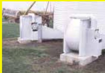
which produces something like 42 btu's of heat per hour. This is heat that would otherwise be lost. We built ductwork around the tops of the fans to suck the air away from around the motors and into the bins. Once you set it up, there's nothing to do. It's money in the bank. **(Irvin Thompson, Seven Hickory Township, Arcola, Ill. 61910 ph 217 268-3293).**
