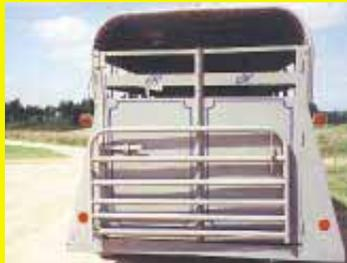
terested in it and how it works. The extra gate mounts on hinges on one side. The other end of the gate hooks onto a bracket on the main door when it's closed. The extra gate helps load animals, yet stays right on the trailer so it's easy to use. **(Kenneth Hubbell, 3141 Goodwill Rd., Hastings, Mich. 49058)**
