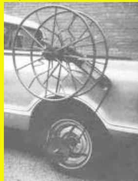
leys and a reel that mounts at one end of a steel shaft that mounts across the width of the pickup bed. The bottom pulley is fastened to a frame that attaches to the pickup wheel rim. The pulley sets out 10 in. from the center of the wheel hub and has adjustable spokes to fit different wheel sizes. A spring-loaded idler arm keeps the belt tight even when you go over bumps.
