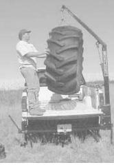
Self-contained hydraulic system uses two hydraulic cylinders. One raises the main mast up to a vertical position; the second raises the lift arm.
