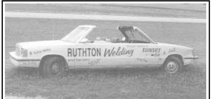
Car has an engine, transmission, and steering wheel at each end. It can be driven in a circle, sideways, or kitty corner, depending on which way the wheels are turned.
