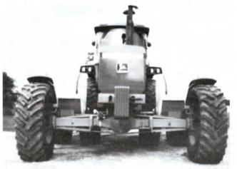
it gave extra room for saddle tanks. I bought some 180-gal. Ag-chem 'tear drop' tanks and saddles but didn't like the position of the tanks. They were too high and too far forward so I built my own brackets. The tanks don't stick out more than 3 or 4 in, past the outside tires with enough room for a cat walk between the tank and the engine, and plenty of room to enter the cab. I moved the latch forward that holds the door open. It now holds the door open so
