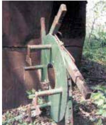
Each spade consists of a length of channel iron with a telescoping length of rectangular tubing inside it. The tubing digs into the ground between the dual wheels.
