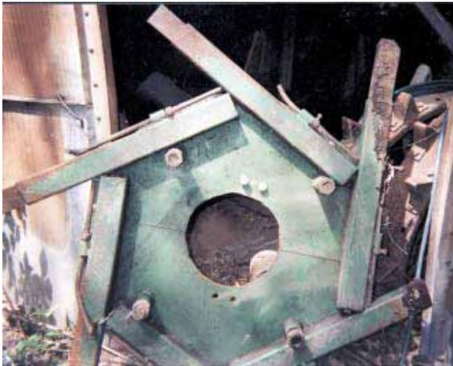
Steel mud spades are welded to a hexagon-shaped steel wheel that bolts to tractor's wheel rim and hub. Each wheel has six mud spades.
