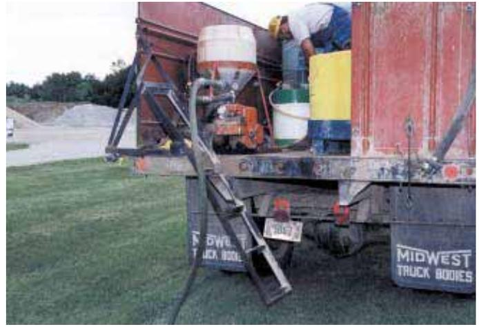
Ladder mounts at right angle to back of truck, making it easy to climb in.
