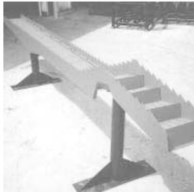
Straw walker bolts on in place of combine's original walker and can be completely closed off or opened to 80 percent. Size of openings is adjusted by using a lever. Photo at left shows entire assembly. Photo on right shows walker open and closed.
