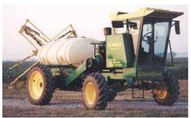
Charlie Zanker started with a 1971 Deere 7100 Turbo combine and ended up with this sleek-looking "SprayBine". It's equipped with a 1,000-gal. tank and 60-ft. boom.
