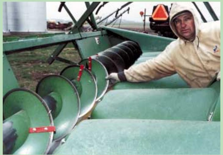
**After equipping his header with a down corn reel, Robert Dunton had trouble with stalks piling up on his feeder auger. To solve the problem, he attached flat metal strips to the edges of flighting.**
