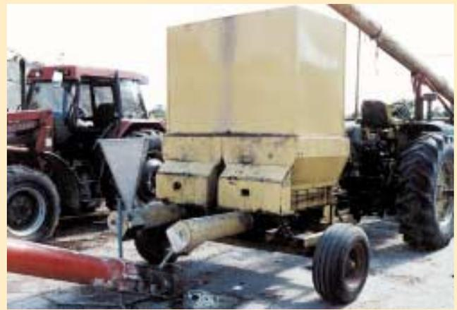
A single hopper feeds grain to the two roller mills, which are mounted together on an axle.
