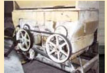
Pto shaft drives pulley on one of the mills, which in turn belt-drives the second mill.
