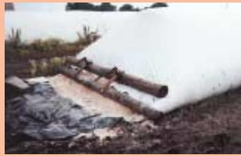
A pair of telephone poles are used to seal open ends of bags. The poles are held together by brackets designed to be picked up by a front-end loader
