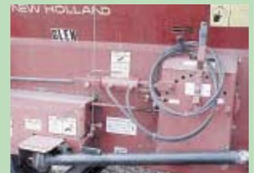
Schweppe attached a double-acting cylinder to the manual speed control lever on his New Holland forage wagon.
