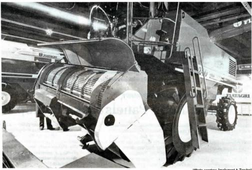
New combine's separator mounts above feederhouse, just behind header (header not shown in photo).
